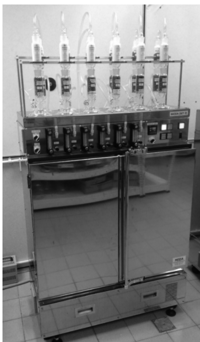
Figure 3. Microbial Oxidative Degradation Analyser (MODA) instrument
